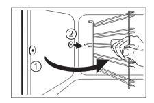
Installing the shelf support rails
